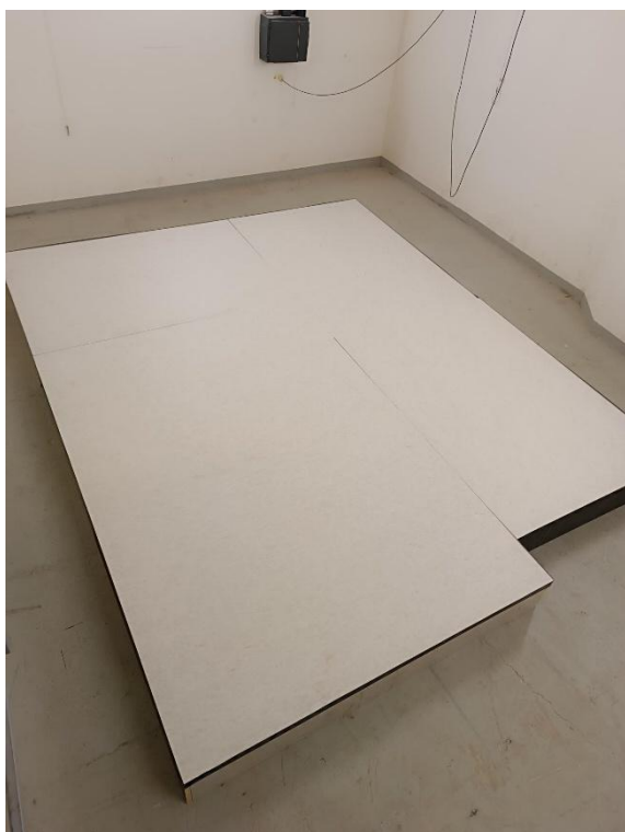
Figure 1: specimen, installed in the reverberation room (ZAG photo archive No. 050037d-04)
