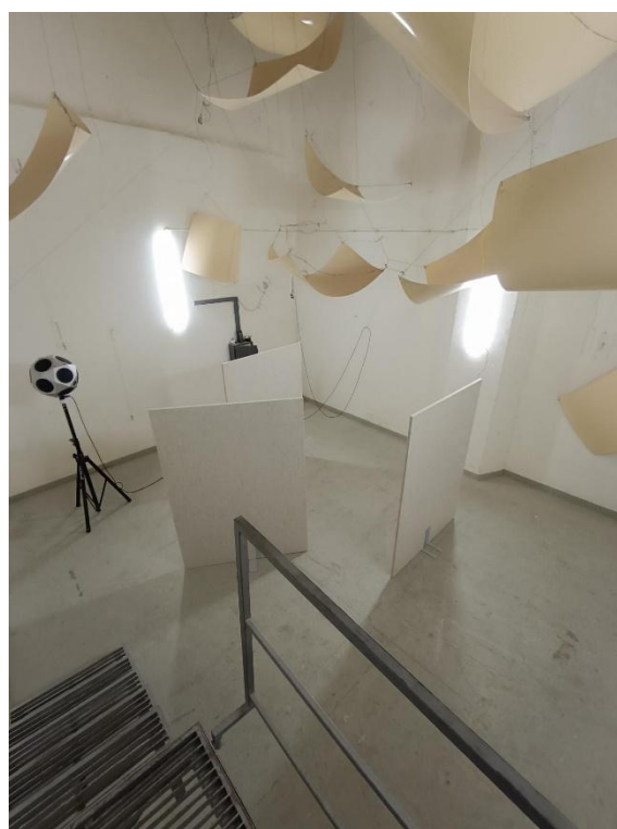
Figure 4: specimen, G mounting in the reverberation room (ZAG photo archive No. 050037d-07)
